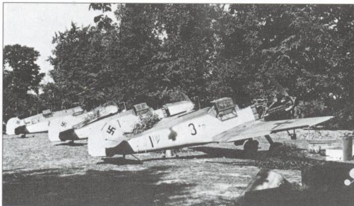
Emils of III./JG 26 undergoing maintenance at Villacoublay in June 1940 after the rigours of the previous weeks' fighting. Note too that the early style narrow-bordered fuselage crosses have been partially oversprayed preparatory to new ones being applied
